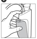
Press Water Tank Release button and remove water tank.
